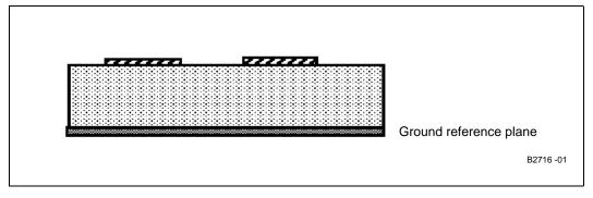
To calculate the coupled impedance requires a 2x2 matrix. The diagonal values in the matrix represent the impedance of the traces to ground and the off-diagonal values provide a measure of how tightly the traces are coupled. The "differential impedance is the value of the line-to-line resistor terminator that optimally terminates pure differential signals." The two by two matrix is shown below as:
